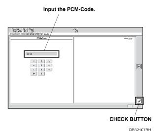
The following message will display: The registration of the Remote Control Engine Starter Unit has been completed. Turn the ignition switch off.
