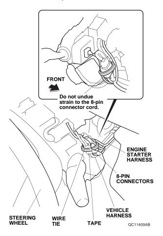
32. Secure the engine starter harness to the vehicle harness with one wire tie.
