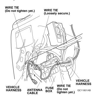
59. Loosely secure the antenna cable to the engine starter harness with one wire tie.
