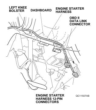
43. Align the white tape on the engine starter harness with the hole on the vehicle bracket, and secure the engine starter harness to the vehicle bracket with one wire tie.
