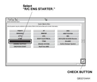
Select REGISTER REMOTE CONTROL ENGINE 7. **STARTER UNIT**, then click the check button.
