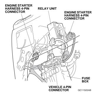
40. Locate the 4-pin connector taped to the vehicle harness, and remove the tape to release the connector. Plug the engine starter harness 4-pin connector into the vehicle 4-pin connector.
