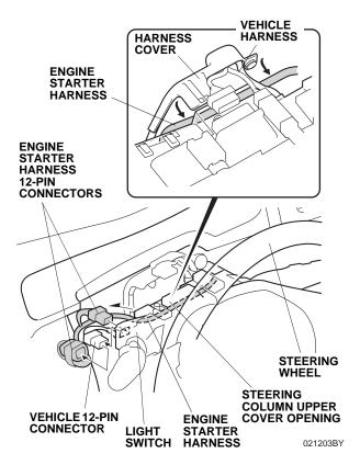
28. Unplug the vehicle 12-pin connector from the light switch, and plug it into the engine starter harness 12-pin connector. Plug the remaining engine starter harness 12-pin connector into the light switch.
