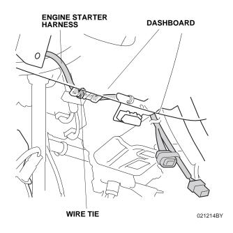
45. Secure the engine starter harness to the ambient light harness with one wire tie.
